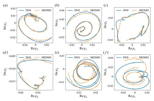
Figure 8. State-space projections of DNS trajectories and their SRDMD approximations from (a-c) the P2K domains and (d-f) the P5K domains, onto complex SRDMD modes centred around the marginal modes. The episodes correspond to (a)  $t \in [240, 300)$ , (b)  $t \in [1280, 1340)$ , (c)  $t \in [1300, 1360)$  in P2K, and  $(d,e) t \in [425, 455)$  and  $(f) t \in [1680, 1710)$  in P5K.
