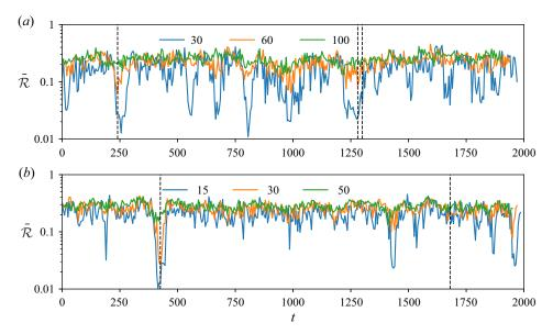
Figure 6. SRDMD residuals (6.1) in (*a*) the P2K domain for time windows of duration  $T_w = 30$ , 60, 100, and (*b*) the P5K domain for  $T_w = 15$ , 30, 50. Time windows were slid across the time series in steps  $\Delta_w = 5$ . Dashed vertical lines correspond to the initial times of the windows that are presented in figures 7–10.
