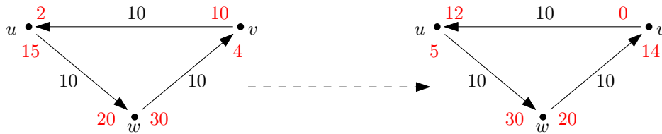
Figure 2.3: The graph on the left depicts three nodes u, v, w connected in a cycle in a PCN. The red numbers by each channel represent the balance of a node in a certain channel. The graph on the right depicts the updated balances of each node on each channel after rebalancing.
