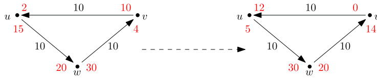
Fig. 2. The graph on the left depicts three nodes u, v, w connected in a cycle. The numbers by each link close to a node represent the capacity of a node in a certain link. u can increase their capacity by 10 on the (u, v) link by first sending the excess capacity of 10 to w along the (u, w) link. Then w sends the excess capacity of 10 to v along (w, v) . Finally, v sends capacity of 10 back to u along (v, u) . The graph on the right depicts the updated capacities of each node on each link after cyclic redistribution.
