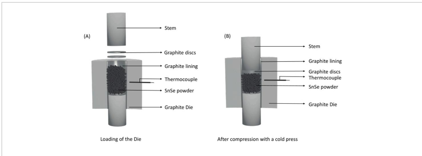
**Figure 2: Illustrations of die preparation for consolidation.** (A) Assembly of the graphite die with the powder. (B) After the powder is compressed using a cold press, the powder is compact, and the total height of the die is reduced to fit between the electrodes. [Please click here to view a larger version of this figure.](#)
