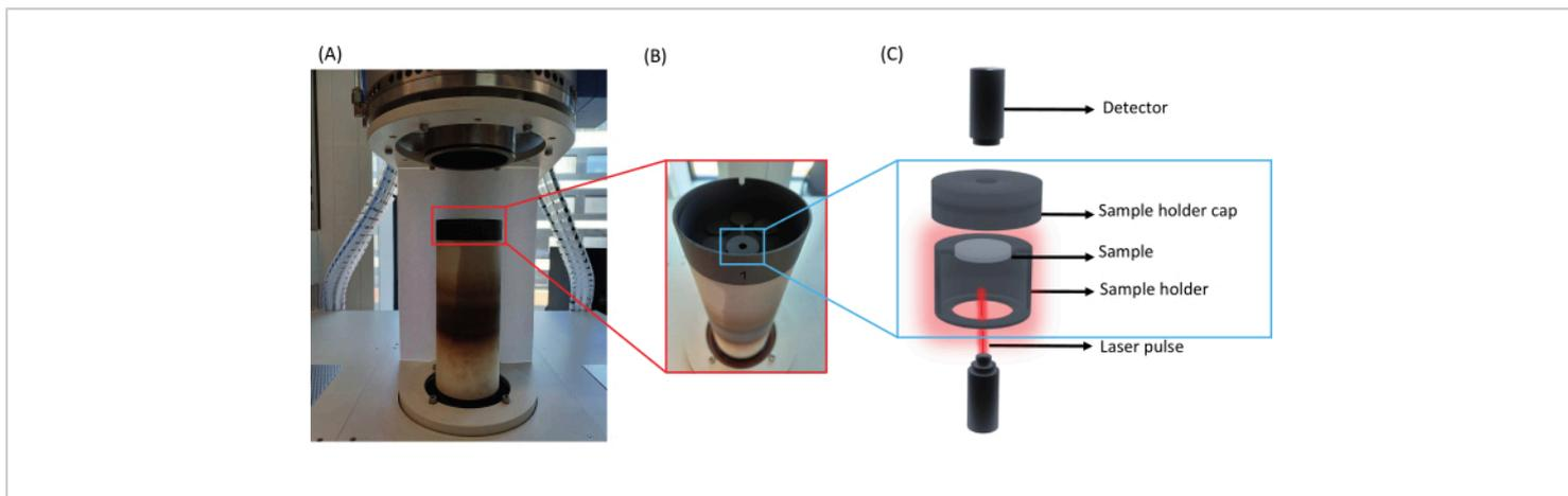
**Figure 4: Thermal diffusivity measurement setup.** (A) Open view of the analyzer, (B) enhanced view of the automated magazine with a sample inside, and (C) schematic illustration of a sample loaded inside a sample holder. [Please click here to view a larger version of this figure.](#)
