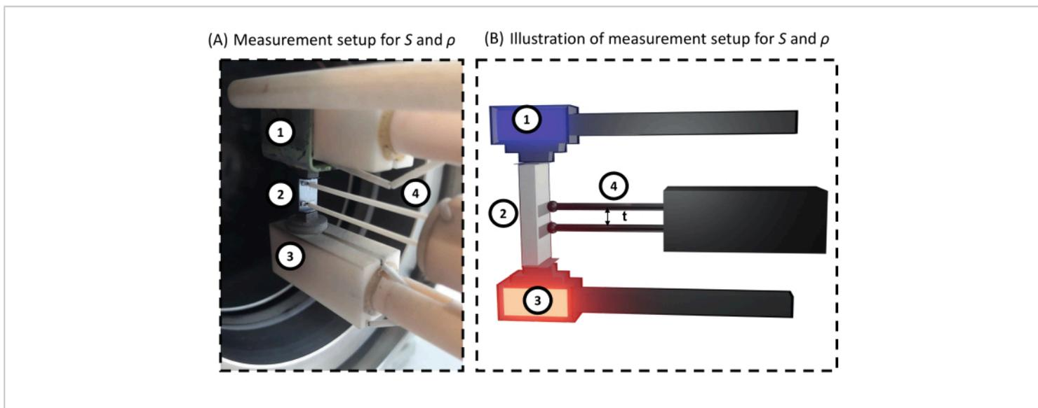
**Figure 3: Measurement setup of the electrical conductivity and the Seebeck coefficient.** For both (A) realistic view of the bar loaded into the device and (B) schematic view; 1) electrode, 2) sample, 3) electrode with gradient heater, and 4) thermocouples/ probes. Between the sample and the electrodes and thermocouples are thin pieces of graphite, aiding the preservation of the device. [Please click here to view a larger version of this figure.](#)
