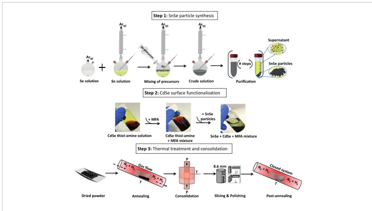
**Figure 1: Steps for the production of CdSe-SnSe pellets divided into three steps:** 1) SnSe particle synthesis, 2) particle surface functionalization with CdSe, and 3) thermal processing into dense CdSe-SnSe pellets. Abbreviation: MFA = *N*-methylformamide. [Please click here to view a larger version of this figure.](#)
