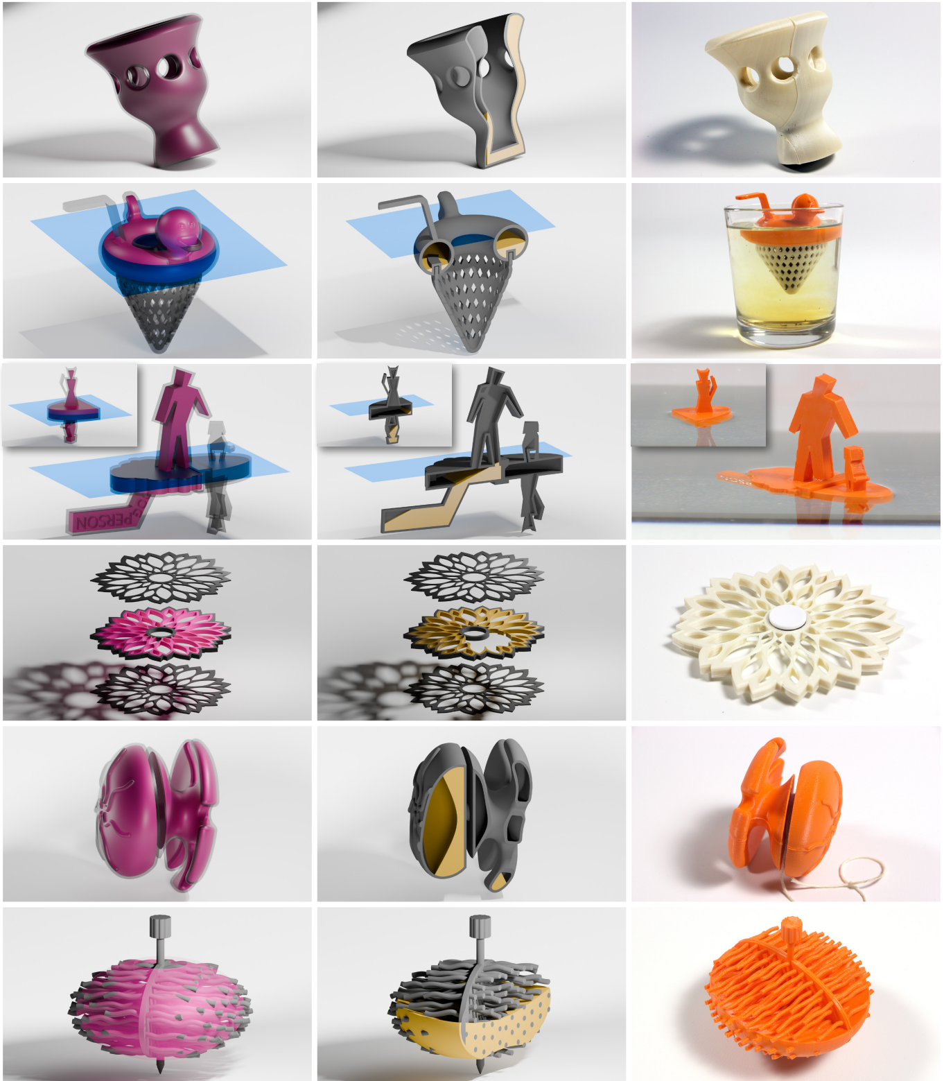
Fig. 9. Optimized Examples. The left column depicts the fixed outer shell in transparent-grey, the design domain in pink, and for the buoyancy examples, the target water line in blue. The middle column shows a cut-away view of the optimized mass distribution in yellow (see Section 6 for the detailed description) and the fabricated objects are represented in the photographs in the right column.
