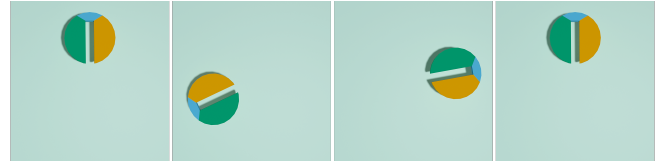
Fig. 13. Zalesak disk. A multi-material test disk rotating around an exterior point without resampling. The disk consists of 108 triangles and fits a 9 \times 9 \times 3 grid region. The whole test runs on a 25^3 grid.
