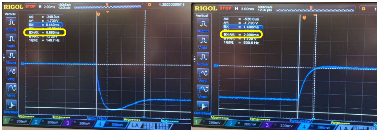
Figure 3.12: Traces of the MOT coil current monitor. The response times are indicated in yellow boxes. Left picture shows the response of turning the MOT current on. It takes about 6.7 ms to turn on with a little transient instability. Right picture shows the response of turning the MOT current off. It takes about 2 ms to turn off with no transient instability.
