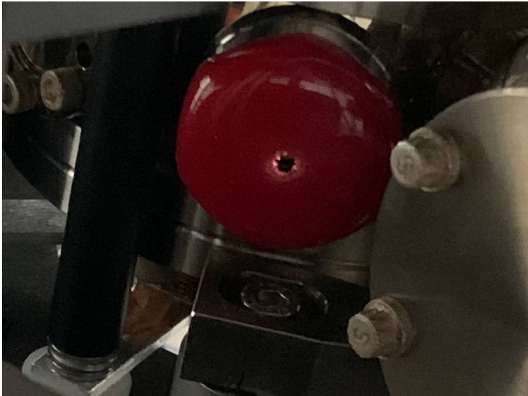
Figure 4.7: Coarse alignment of 3D MOT beams using the rubber caps on the view ports. Since we can not use other alignment procedure this helped us recover the 3D MOT after completely loosing it.
