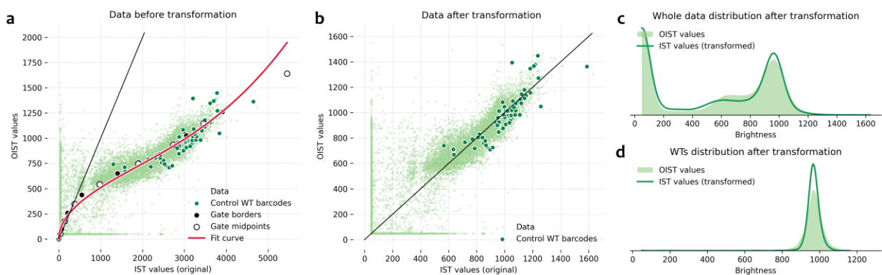
FIGURE 42. Merging of data from two FACS runs. Data from cgreGFP:1338 is shown, as an example. (a) Data from IST and OIST runs, prior to rescaling; X and Y axes show respective fluorescence values. Light green points represent all barcodes with cell counts over 15 measured in both experiments. FACS gate borders (black dots), gate midpoints (white dots), and control barcodes from 17 cgreGFP -derived “WTs” (dark green dots) are also shown. For reference, the black line, f(x) = x , shows ideal fluorescence agreement between the two experiments. All data points represented were used to fit the red curve, f(x) = a \cdot x^b + c \cdot x . (b) Data points as in (a), after transforming the IST values according to the parameters of the fitted curve and applying a linear rescaling to align the minimal and WT fluorescence values. Again for reference, the black line shows f(x) = x . (c) Distribution of the IST (dark green outline) and OIST (light green fill) library data, after rescaling. (d) As (c), but showing only WT genotypes.
