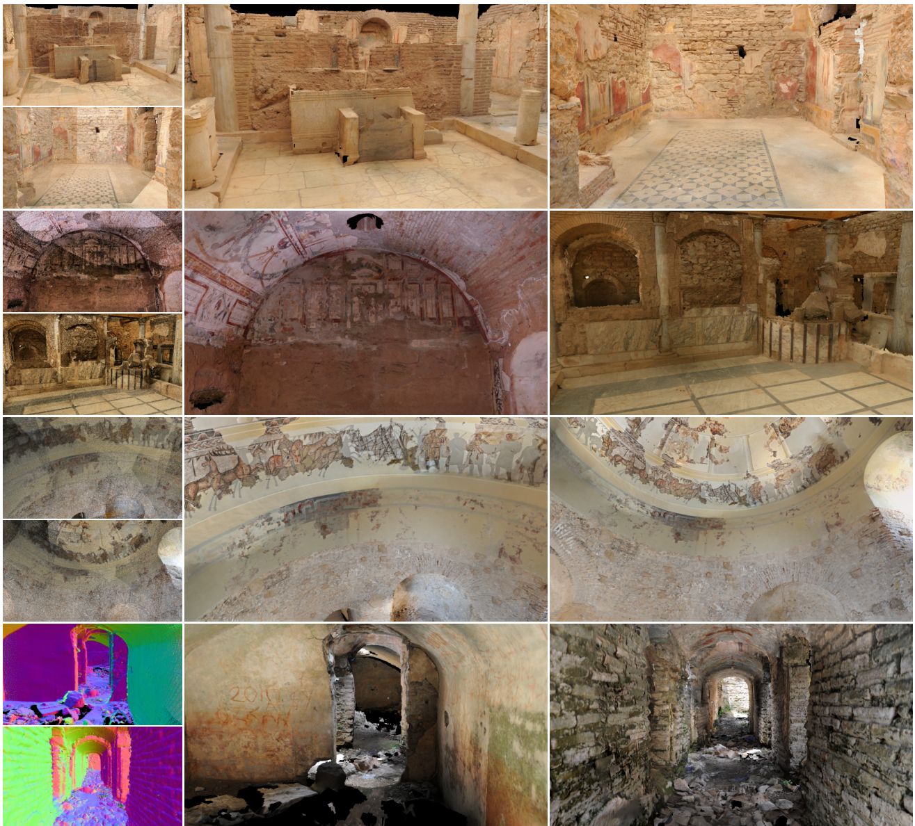
Fig. 14. Two views of each input point cloud, and the corresponding multi-mesh representations of (from top to bottom) Hh2 We1 , Hh2 We6 , Centcelles and 7schläfer datasets. The point clouds are displayed with the colors acquired by a scanner. In the last example, points are color-coded according to their normals.
