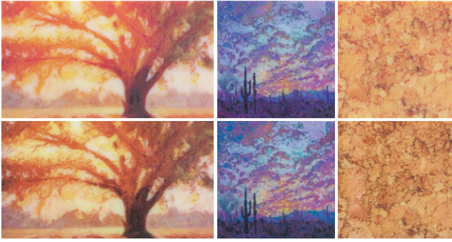
Fig. 18. A subset of our samples illuminated by direct sunlight on a clear day, comparing the unsharp-masked default prints ( top row ) with our optimized results ( bottom row ). The light is arriving from the top-right, with the zenith angle of approximately 50^\circ . Although our results are not optimized for such directionally non-uniform light, their structure is preserved comparatively better (cf. respective targets in Fig. 17).
