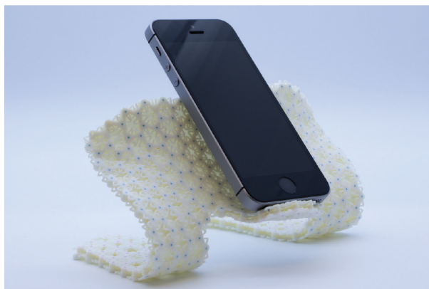
Figure 1.5: Our shells have remarkable load bearing capabilities. We designed a mobile phone stand holding an item twice its own weight.
